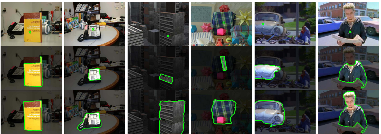
Fig. 15. Columns 1-3: A moving camera and stationary objects. Column 4: An image from a stereo pair. Column 5: A moving object (car) and a stationary camera. Column 5: Moving objects (human, cars) and a moving camera. Row 1: The original images with fixations (the green "X"). Row 2: The segmentation results for the fixation using static cues only. Row 3: The segmentation for the same fixation after combining motion or stereo cues with monocular cues.
